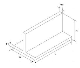
Cross-section Dimensions (in mm) W: 10, 15, 20, 25, 30, (40) H: 10, 15, 20, 25, 30, (40) T1: 1.5 to 3.0 T2: 1.5 to 3.0
